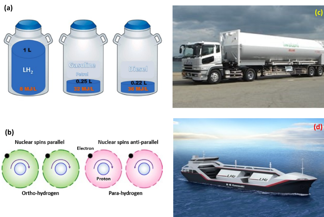
Figure 4: (a) Graphical comparison of energy content per unit volume based on the lower heating values (LHV) of the fuels (Morales-Ospino et al. 2023); (b) the direction of parallel and antiparallel nuclear spins of hydrogen molecules (Ghorbani et al. 2023). Reproduced with permission from Elsevier; Hydrogen transportation examples: (c) Iwatani Corporation \text{LH}_2 transport container (Kawasaki 2025), and (d) Ship Carrying Liquefied Gases in Bulk (total carrying capacity: 2,500 \text{m}^3 ) (Kawasaki 2014).
