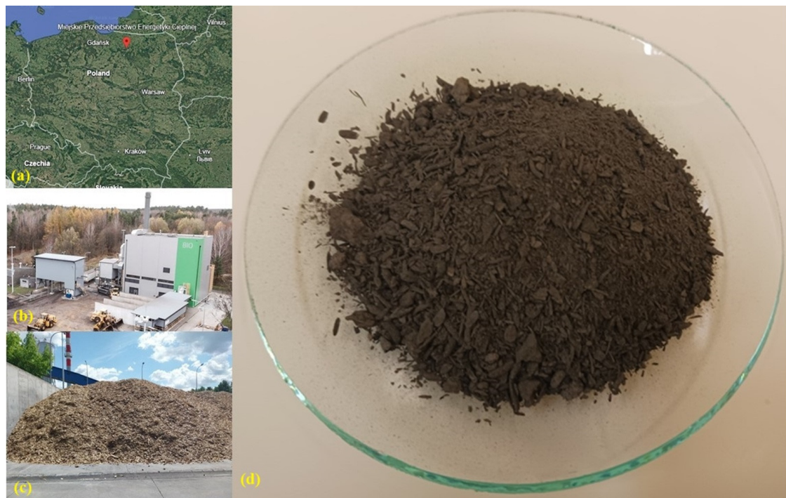
Figure 1. (a) Location of the Municipal Heating Energy Company in Olsztyn (MPEC Olsztyn, Poland); (b) heating energy facility where biomass combustion and ash generation occur; (c) wood chips used as fuel; (d) WBA obtained as the combustion by-product.
